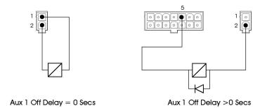
The output will be active depending on how the parameter Auxiliary 1 Output Mode is programmed. The three modes, which should be used to control an auxiliary motor, are Forward Traction, Reverse Traction or Traction.
