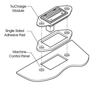
When correctly fitted, this arrangement will give the TruCharge Module an IPX5 ingress protection rating.
