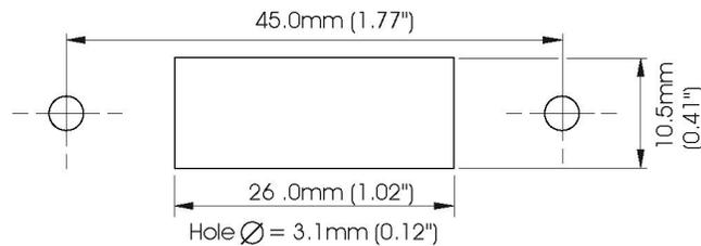
Alternatively M3 (4-40 UNC) hardware can be used. The height of the display from the printed circuit board is 8.0mm (0.31 inches). Suitable spacers should be used so that the display is fixed slightly below the machine's control panel. Ensure that the metallic fixing hardware (nuts, washers etc.) do not touch the conductive tracks on the printed circuit board.
