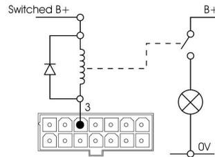
If the current drawn is less than the value shown in the preceding table, the relay is not required and the lamp can be connected directly between Switched B+ and pin 3
