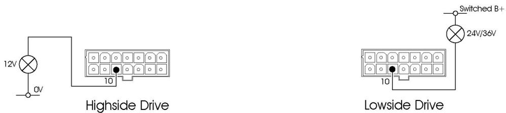
If you are using an LED, it is connected between the same points but you must provide a series connected current limiting resistor.
