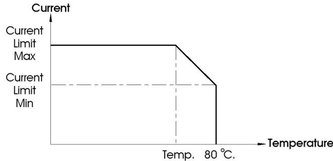
If the i-Drive's internal temperature reaches the value set by Current Foldback Temperature, the maximum current output will be reduced from the value set by Current Limit Max. The reduction will be linear to a value set by Current Limit Min. at a fixed internal temperature of 80°C.
