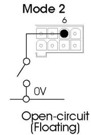
The parameter can be set to Disabled, Pull Low or Open Circuit.
