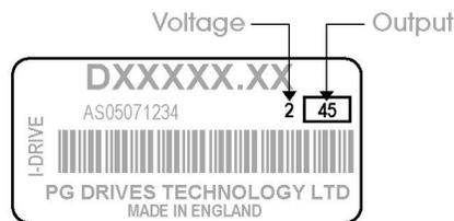
The number in the box indicates the output current; the single digit number to the left of the box indicates the operating voltage.
