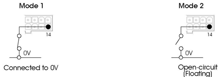
The parameter can be set to Disabled, Pull Low or Open Circuit.
