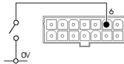
Each Inhibit input has been designed to either inhibit a specific function or control an auxiliary function such as a brush or vacuum motor. The Inhibits can be used to either limit the maximum speed of the machine, stop it completely or in the case of an auxiliary output, stop and start the output device.
