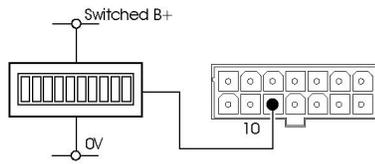
If you are using a bulb, the bulb can be connected directly between pin 10 and 0V (Highside) or pin 10 and switched B+ (Lowside). The bulb must be 12V with a maximum rating of 600mW when connected Highside and 24V / 36V with a maximum rating of 600mW when connected Lowside.
