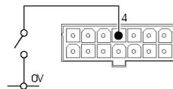
If pin 4 is connected to 0V the controller will drive using the programmed slow speed and rates. These speeds are listed below.
