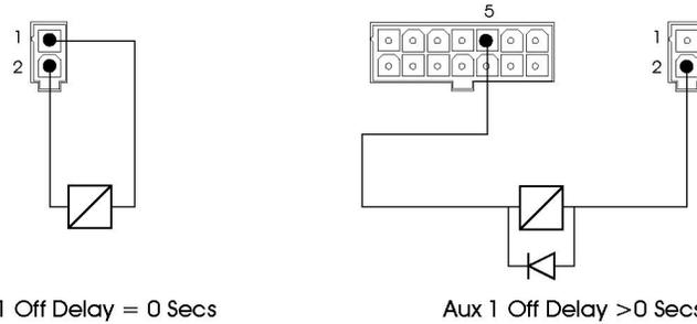
The output will be active depending on how the parameter Auxiliary 1 Output Mode is programmed. The three modes, which should be used to control an auxiliary motor, are Forward Traction, Reverse Traction or Traction.
