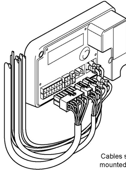
Cables should be mounted as shown
