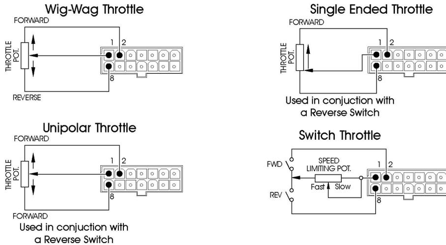
If a switch operated throttle is required, the parameter Throttle Type must be set to Wig-wag and the parameter Throttle Reference Test must be set to Off.
