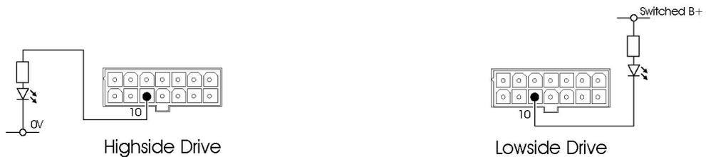
If you are using an Analogue 12V Status Indicator, it must be connected between pin 10 and 0V.
