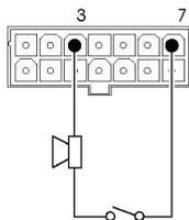
To enable this function, Auxiliary 2 Output Mode should be set to Diagnostic/Reverse Alarm.
